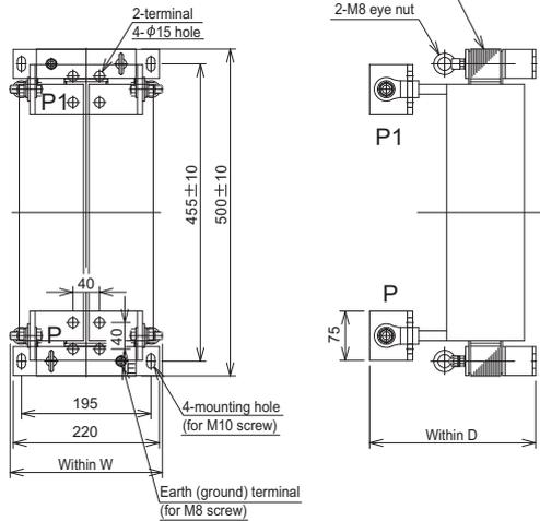
\* Remove the eye nut after installation of the product.
