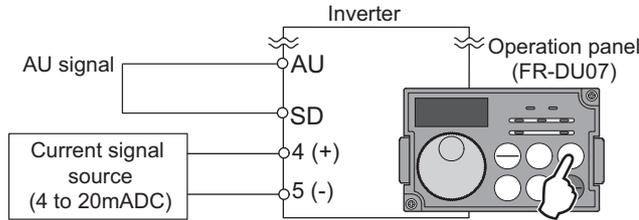
**Operation example** Performing operation at 60Hz.
