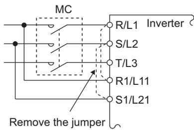
When a fault occurs, opening of the electromagnetic contactor (MC) on the inverter power supply side results in power loss in the control circuit, disabling the fault output signal retention. Terminals R1/L11 and S1/L21 are provided to hold a fault signal. In this case, connect the power supply terminals R1/L11 and S1/L21 of the control circuit to the input side of the MC. Do not connect the power cable to incorrect terminals. Doing so may damage the inverter.
