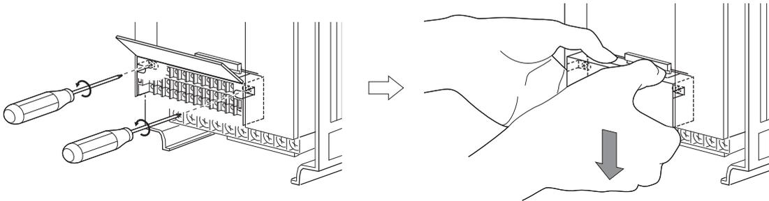
2) Change the jumper connector set to the sink logic (SINK) on the rear panel of the control circuit terminal block to source logic (SOURCE).
