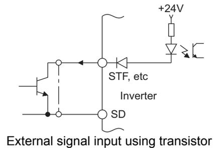
External signal input using transistor
