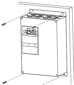
Fix six positions for the FR-A740-160K to 355K and fix eight positions for the FR-A740-400K to 500K.
