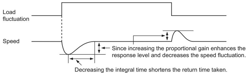
$$\text{Actual speed gain} = \text{speed gain of motor without load} \times \frac{JM}{JM+JL}$$
