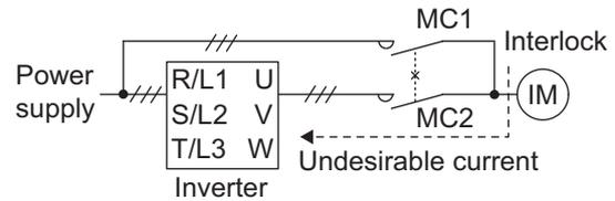
**(14) If the machine must not be restarted when power is restored after a power failure, provide a magnetic contactor in the inverter's input side and also make up a sequence which will not switch ON the start signal.**
