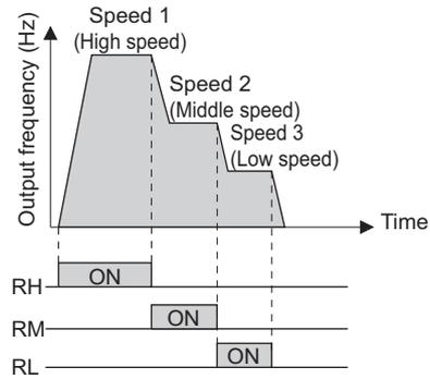
Changing example Operation at high speed (60Hz).
