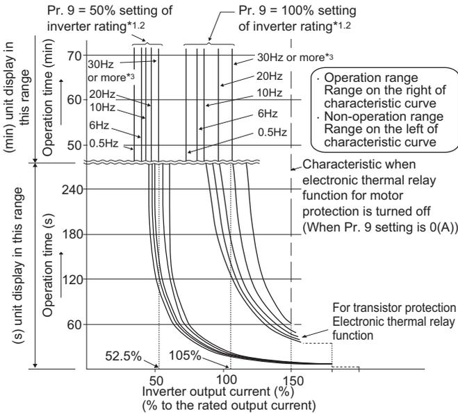
This function detects the overload (overheat) of the motor, stops the operation of the inverter's output transistor, and stops the output.
