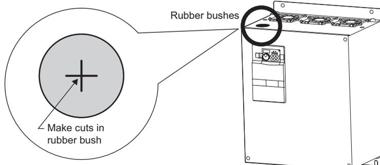
2) Insert a connector on the MT-BU5 side through a rubber bush to connect to a connector on the inverter side.
