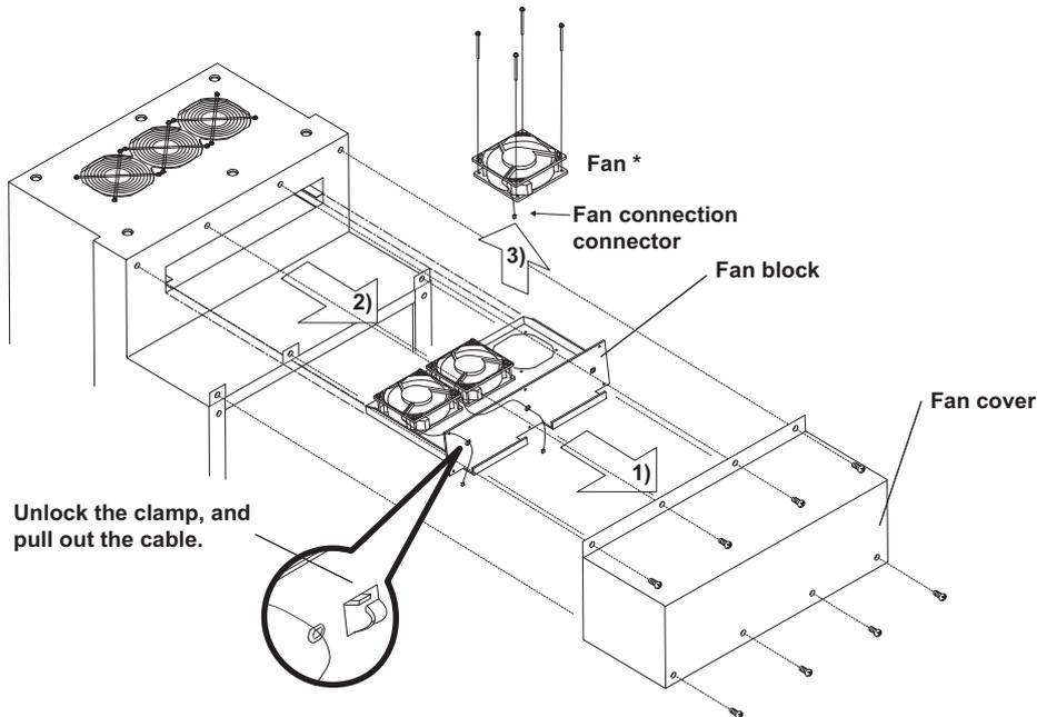
\* The number of cooling fans differs according to the inverter capacity.
