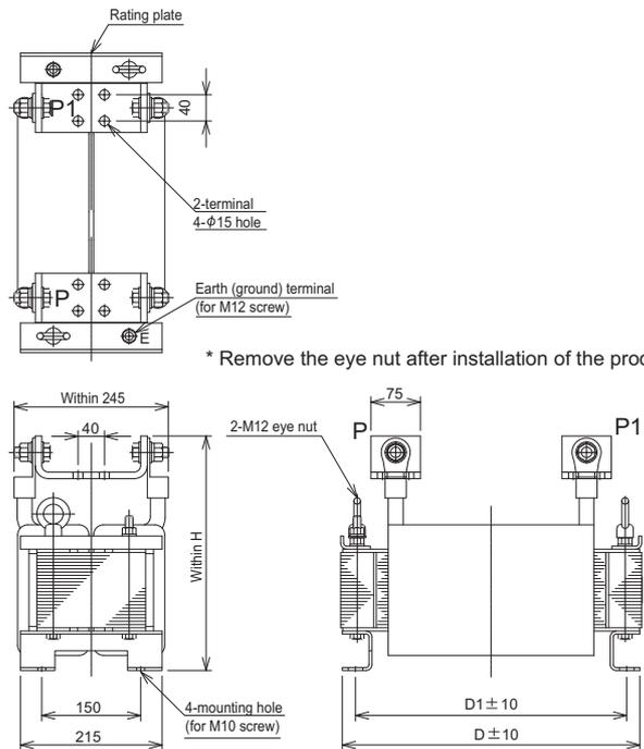
\* Remove the eye nut after installation of the product.
