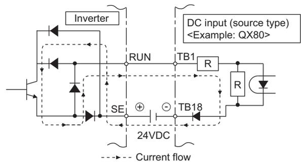
• When using an external power supply for transistor output
