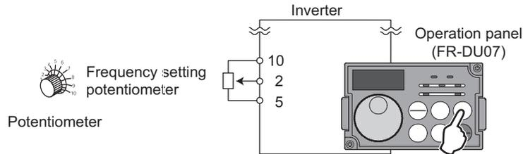
**Operation example** Performing operation at 60Hz.
