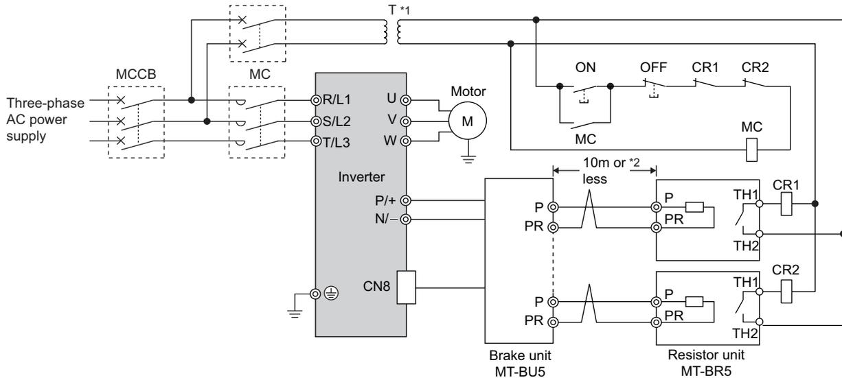
\*1 When the power supply is 400V class, install a stepdown transformer.
