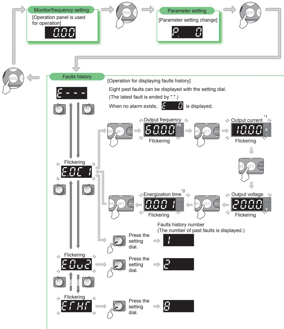
\*1 When an overcurrent trip occurs by an instant overcurrent, the monitored current value saved in the faults history may be lower than the actual current that has flowed.
