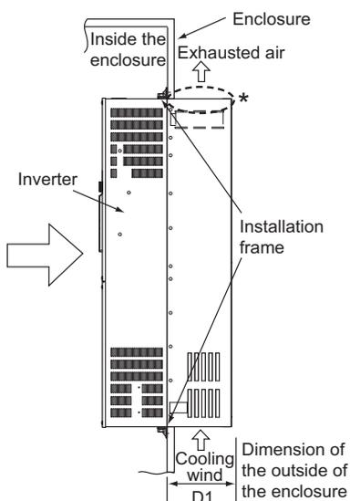
\* For the FR-A740-160K or higher, there are finger guards behind the enclosure. Therefore, the thickness of the panel should be less than 10mm (\*1) and also do not place anything around finger guards to avoid contact with the finger guards.
