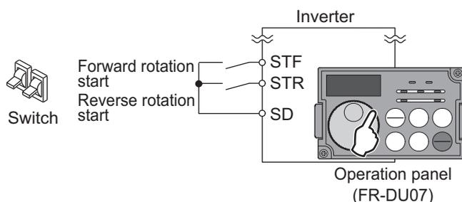
Operation example Performing operation at 30Hz.
