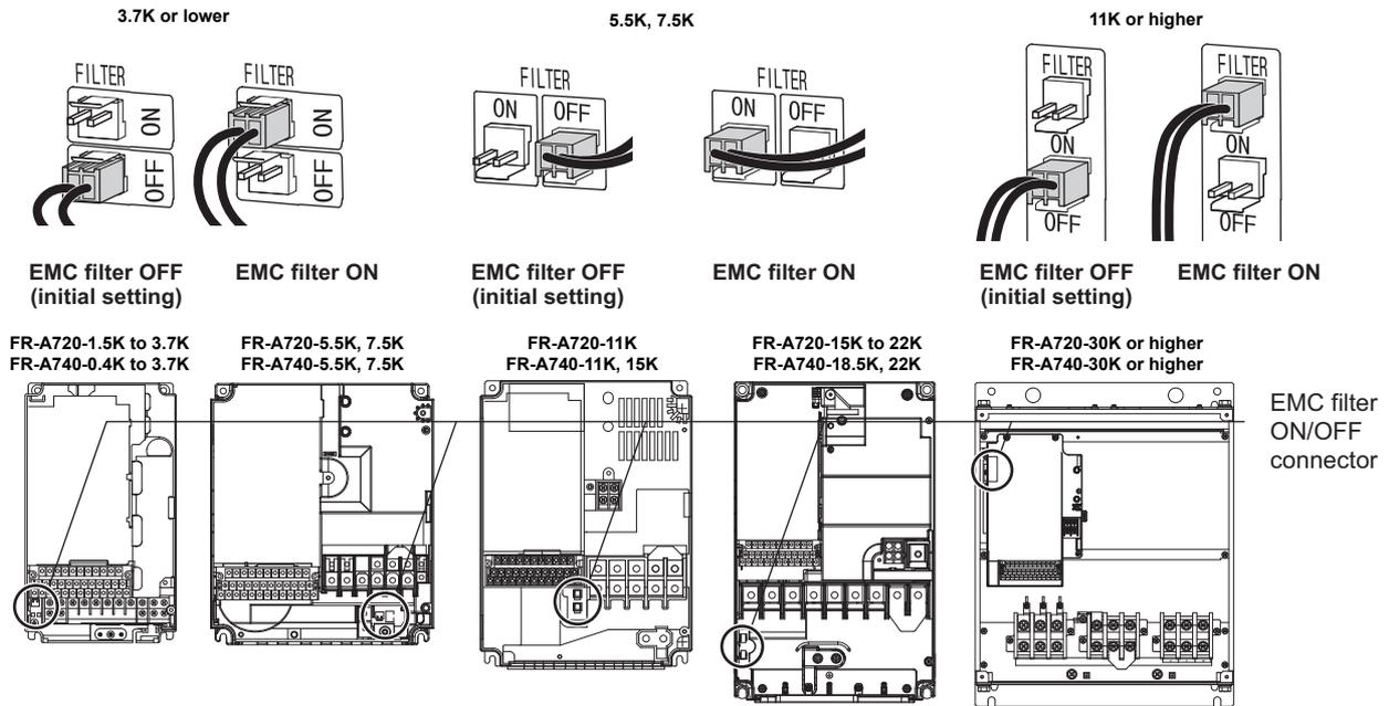
The FR-A720-0.4K and 0.75K are not provided with the EMC filter ON/OFF connector. (The EMC filter is always valid.)
