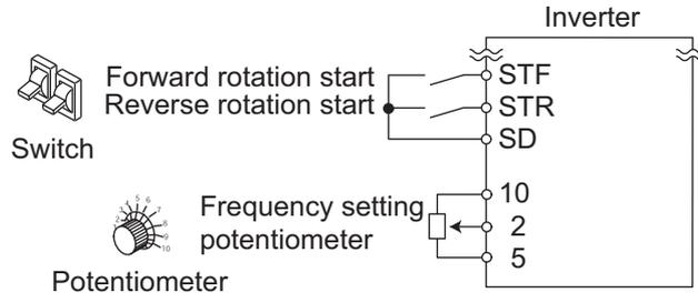
**Operation example** Performing operation at 60Hz.
