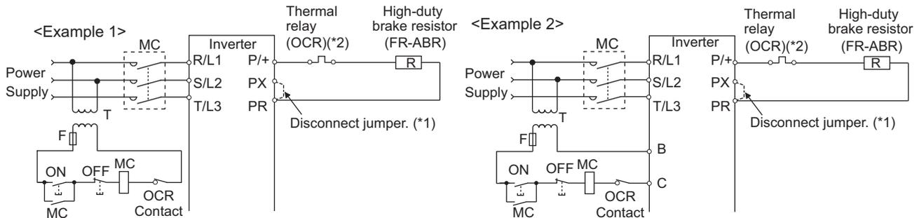
\*1 Since the 11K or higher inverter is not provided with the PX terminal, a jumper is not need to be removed.
