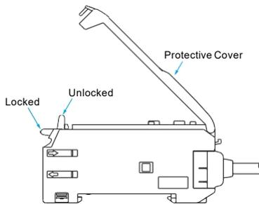
**Note:** To maintain the fiber unit properties, confirm that the lock is released before removing the fiber unit.
