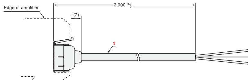
\* E3X-CN11: 4 dia. cable / 3 conductors / Standard length: 2 m (Conductor cross section: 0.2 mm<sup>2</sup> (AWG24), Insulator diameter: 1.1 mm)
