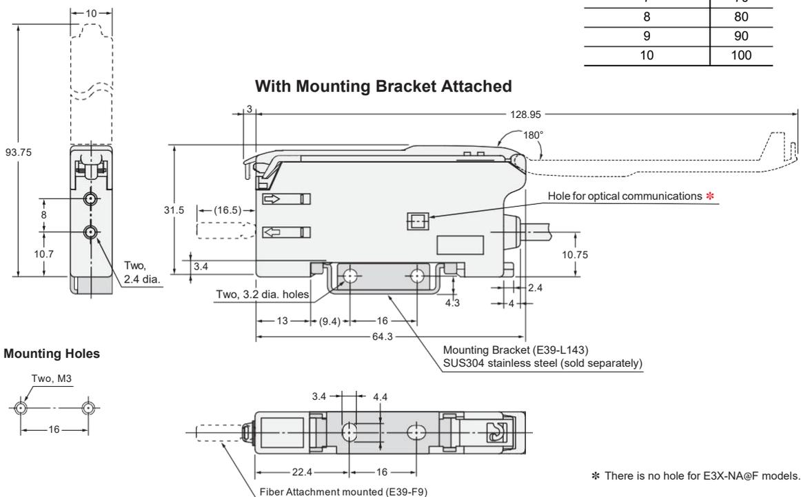
**Note:** When using E39-L143 Mounting Brackets, there will be small gaps between the Fiber Amplifier Units if they are mounted side by side.
