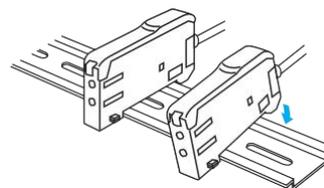
2. Slide the Amplifier Units together, line up the clips, and press the Amplifier Units together until they click into place.
