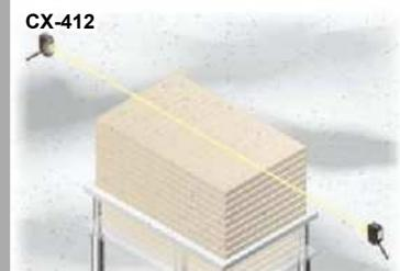
**Passage confirmation of object on a conveyor belt**
