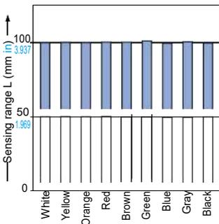
These bars indicate the sensing range with the respective colors when the distance adjuster is set to a sensing range of 100 mm **3.937 in** and 50 mm **1.969 in** long, respectively, with white color. The sensing range also varies depending on material.
