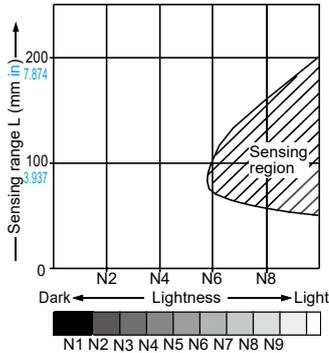
The sensing region is represented by oblique lines in the left figure. However, the sensitivity should be set with an enough margin because of slight variation in products.
