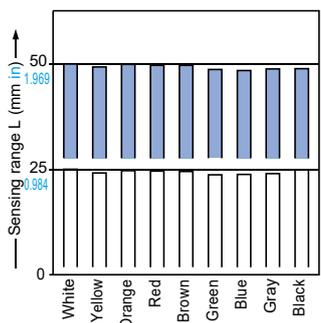
These bars indicate the sensing range with the respective colors when the distance adjuster is set to a sensing range of 50 mm 1.969 in and 25 mm 0.984 in long, respectively, with white color. The sensing range also varies depending on material.
