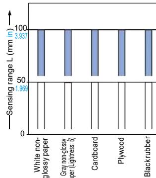
These bars indicate the sensing range with the respective objects when the distance adjuster is set to a sensing range of 100 mm **3.937 in** and 50 mm **1.969 in** long, respectively, with white non-glossy paper.
