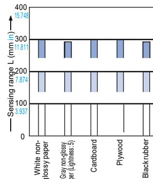
These bars indicate the sensing range with the respective objects when the distance adjuster is set to a sensing range of 300 mm **11.811 in**, 200 mm **7.874 in** and 100 mm **3.937 in** long, respectively, with white non-glossy paper.
