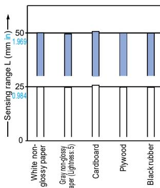
These bars indicate the sensing range with the respective objects when the distance adjuster is set to a sensing range of 50 mm 1.969 in and 25 mm 0.984 in long, respectively, with white non-glossy paper.
