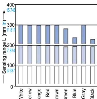
These bars indicate the sensing range with the respective colors when the distance adjuster is set to a sensing range of 300 mm **11.811 in**, 200 mm **7.874 in** and 100 mm **3.937 in** long, respectively, with white color. The sensing range also varies depending on material.
