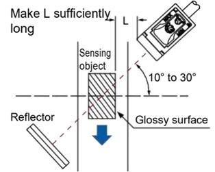
**Retroreflective type sensor with polarizing filters (CX-491)**
