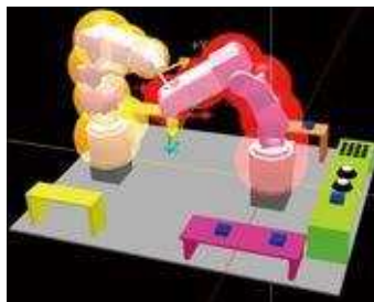
Checking interference using the robot with a defined solid model
